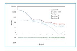
Transmission SAXS from nanoparticles suspended in solution is a powerful method for the determination of particle sizes and shapes. The requirement for accurate size and shape information is important in many of the emerging areas of nanomaterials research currently taking place throughout the world. The Ultima IV with CBO offers one touch switching from conventional wide angle scattering and diffraction geometries to the ultra-low angle performance needed for SAXS measurements.
