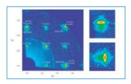
Perhaps the most useful measurement for the rigorous interpretation of thin film properties by X-ray diffraction is the reciprocal space map (RSM). RSMs show both the location and characteristics of reciprocal space points coming from epitaxial heterostructures. RSMs can be used to interpret orientation, perfection, strain, and relaxation in complex materials. In this example, the use of in-plane scanning allows information to be gathered in directions parallel to the thin film sample surface.
