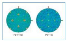
For thin film materials, pole figure analysis can be used to determine orientation relationships between substrates and deposited materials. In this example, in-plane pole figures were collected on both the Pt substrate and (Pb, La)TiO<sub>3</sub>/Pt/MgO PLT thin layer. The epitaxial relationship between the substrate and layer material is clearly shown. Critical to this measurement is the in-plane geometry, which allows full pole figures to be collected on both the substrate and the thin layer.
