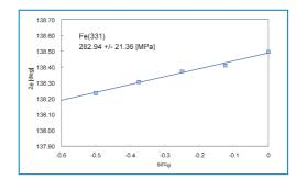
For residual stress measurements the determination of absolute peak positions is crucial. Since peak positions are strongly affected by sample displacement errors, CBO and automatic sample alignment are critical to both accurate results and ease of measurement. The figure to the left shows a traditional  $\sin^2\!\Psi$  plot from an iron nut. This odd shaped sample is easily aligned and accurately measured using the Ultima IV configured with CBO.
