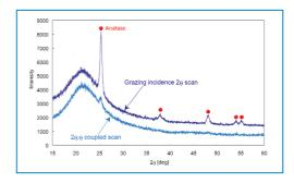
The use of glancing incidence scanning is shown to be critical in this measurement of a photocatalyst thin film. CBO allows the measurement of thin films easily and in complement to other bulk materials and powders. The figure to the left shows the enhancement of the diffraction data in glancing incidence mode compared to a conventional  $\theta/2\theta$  symmetric measurement. Diffraction peaks from the film are clearly visible in glancing incidence mode.
