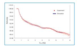
X-ray reflectivity (XRR) measurements are used to determine thin film thickness, surface roughness, interface roughness, and density in layered materials. Again, the one touch selection of parallel beam geometry provided by CBO, and automatic sample alignment critical to XRR, makes performing these measurements simple. The example to the left shows both the calculated and experimental collected XRR curves from a three layer stack of oxidized GaAs, GaAs, InGaAs on a GaAs substrate.
