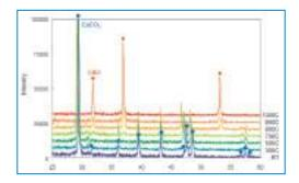
Collecting XRD data at variable temperatures can provide structural information on materials under conditions similar to those in which the material will ultimately be used. In this example, the Ultima IV with CBO in focusing mode coupled with a fast position sensitive detector is used to collect high-speed (two minutes per scan) diffraction data from a CaCO<sub>3</sub> sample undergoing a thermally induced reaction to CaO. The transition to CaO can be seen to occur at approximately 800°C.
