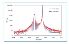
For high-resolution X-ray diffraction, the CBO module provides a high-quality, intense, parallel beam for further conditioning by the automatically aligned multiple crystal optics, proving optimal performance from a simple-to-use configuration. A high-resolution rocking curve (left) shows peak separation between the layer and substrate reflections, giving alloy composition.
