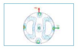
On-demand in-plane scanning provides the ultimate in flexibility when collecting pole figure data. In this example, pole figure data collected from a Cu (111) plate using in-plane geometry extends out to the edge of the pole figure plot. It was not necessary to re-configure the system to point focus mode or re-mount the sample for transmission measurement to collect this "full",  $\alpha=0$  to 90°, pole figure.
