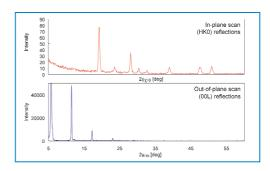
On-demand, combined in-plane and out-of-plane scanning provides a full picture of the texturing in thin films. In this example, in-plane (00L) and out-of-plane (HK0) scans were made on a 50 nm Si/pentacene thin film structure. The in-plane measurement done at a 0.18° glancing incident angle provides a unique look at the orientation of the film.
