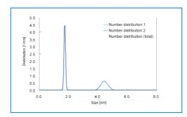
In this example, the experimental SAXS curve (above left) has been overlaid with the calculated SAXS curves from a bimodal distribution of particle sizes (left) modeled in NANO-Solver, Rigaku's powerful software solution for SAXS data processing. The agreement between the experimental and calculated curves shows that the proposed distribution model is in good agreement with what is actually contained in the sample, as observed by TEM.
