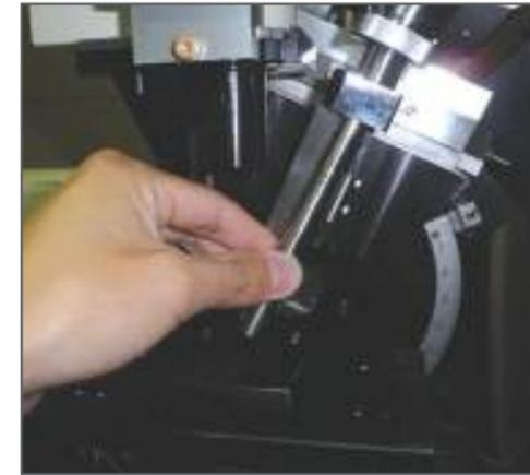
Residual stress in a micro area is measured by utilizing optional collimators. The collimators are easy to install and remove. Optional sizes are:  $\phi 30 \mu\text{m}$ ,  $\phi 50 \mu\text{m}$ ,  $\phi 100 \mu\text{m}$ , as well as  $\phi 300 \mu\text{m}$ ,  $\phi 500 \mu\text{m}$ ,  $\phi 2 \text{ mm}$ , and  $\phi 4 \text{ mm}$ . Standard collimator sizes are  $\phi 150 \mu\text{m}$  and  $\phi 1 \text{ mm}$ .
